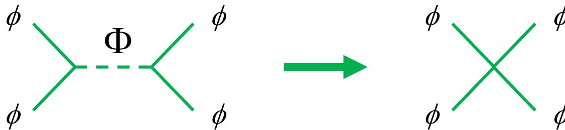
$$\mathcal{A}_{\text{UV}} \sim \frac{1}{\hat{s} - M^2} \quad \mathcal{A}_{\text{EFT}} \sim -\frac{1}{M^2} \left[ 1 + \frac{\hat{s}}{M^2} + \left( \frac{\hat{s}}{M^2} \right)^2 + \left( \frac{\hat{s}}{M^2} \right)^3 + \dots \right]$$
