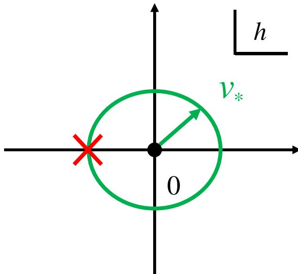
$$|\partial_h^n \mathcal{K}_h| \sim \frac{n!}{v_*^n} \quad \text{Cauchy-Hadamard theorem}$$
